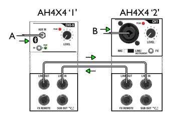
When using the 'Link In' socket, sleep mode is temporarily disabled so that the slave does not shut down un-necessarily. (Sleep mode monitors the input channels)
